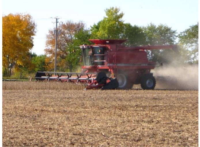
Figure 3. Harvest losses due to lodged soybean plants can be minimized with careful combine adjustments and operation.
